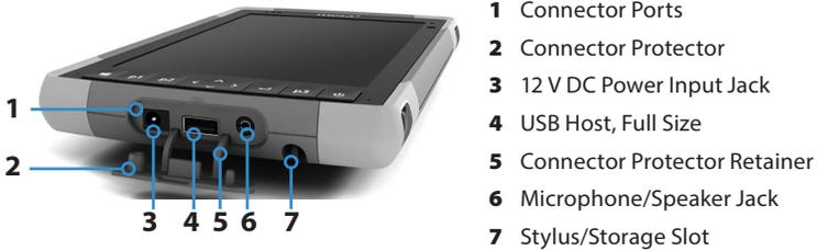
The connector protector is removable and replaceable. See your sales representative for if you need a new one. To remove it, pull it out of the ports, then gently pull the curved rubber retainers out of the holes they are in. Replace it by inserting the curved rubber retainers back into the holes.
