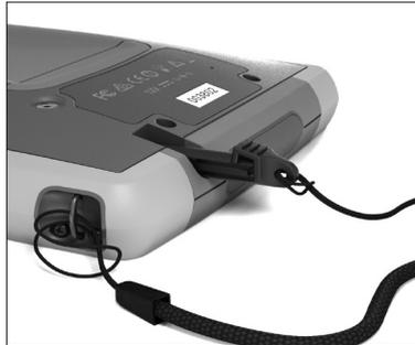
3. Insert the stylus with the attached tether through this loop and tighten the loop.
