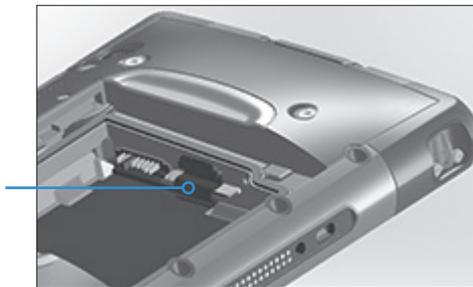
5. Push the flexible card holder back into place, covering the card slots.
